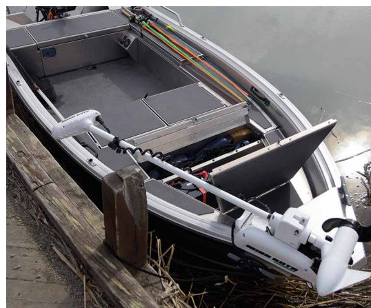
Casting deck for bow and motor bracket
