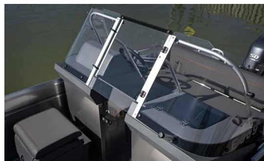
The fixed door between the consoles protects from wind and spray.
