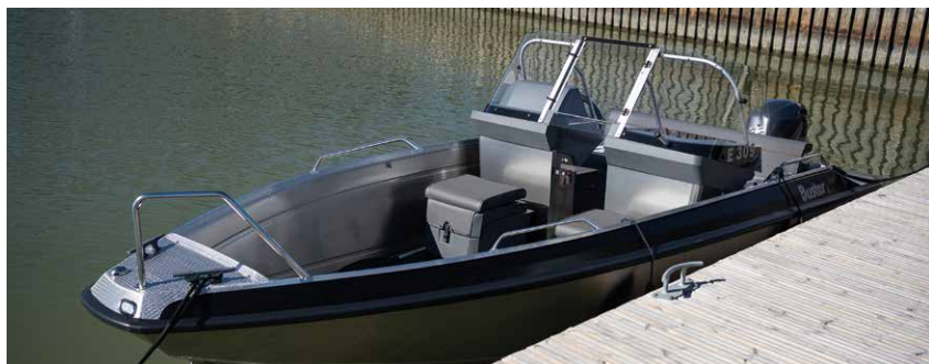
Flexible general arrangement due to the removable seat/stowage boxes
